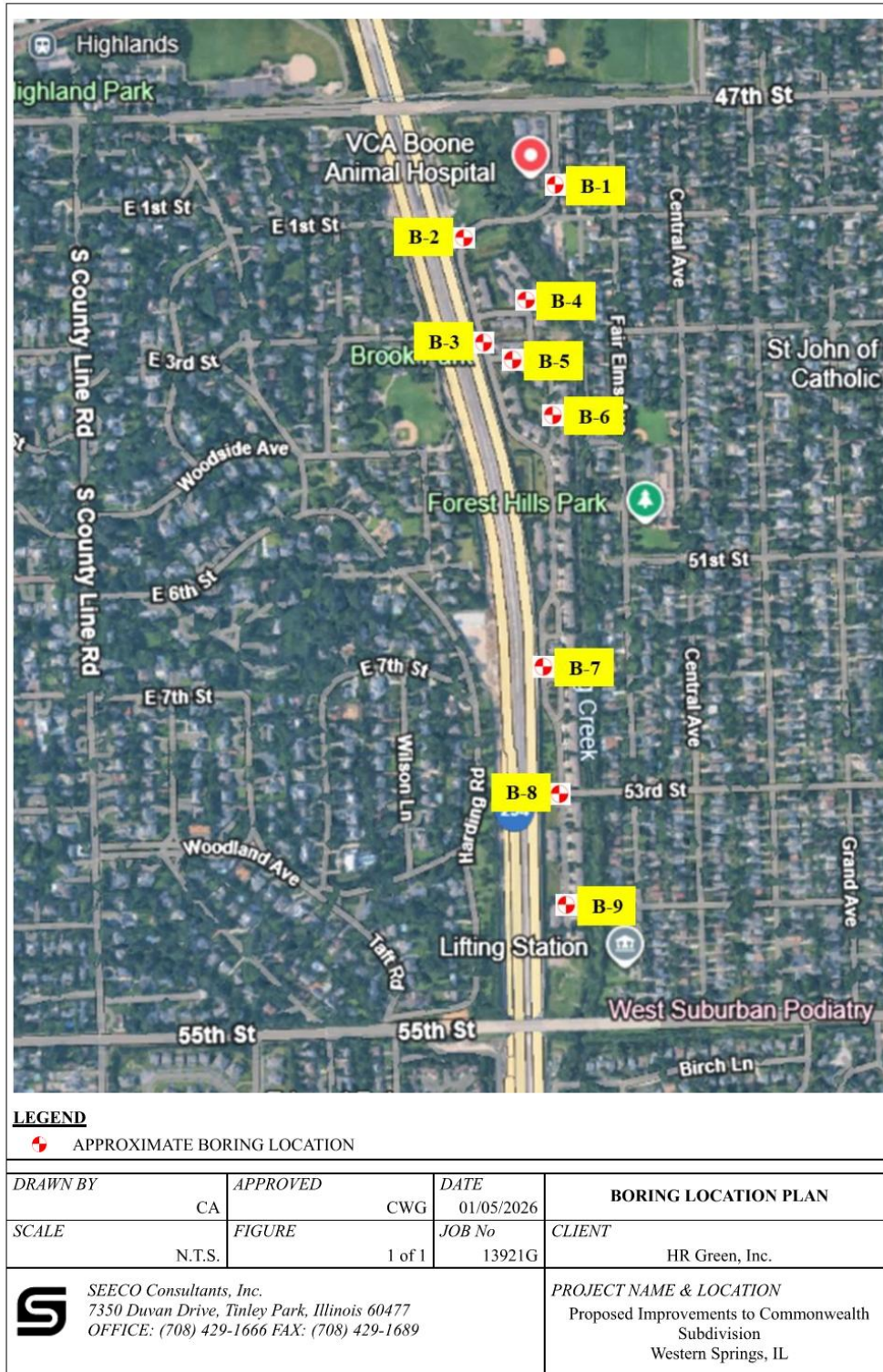
Figure 1: Boring Location Map (from Geotech Report)
