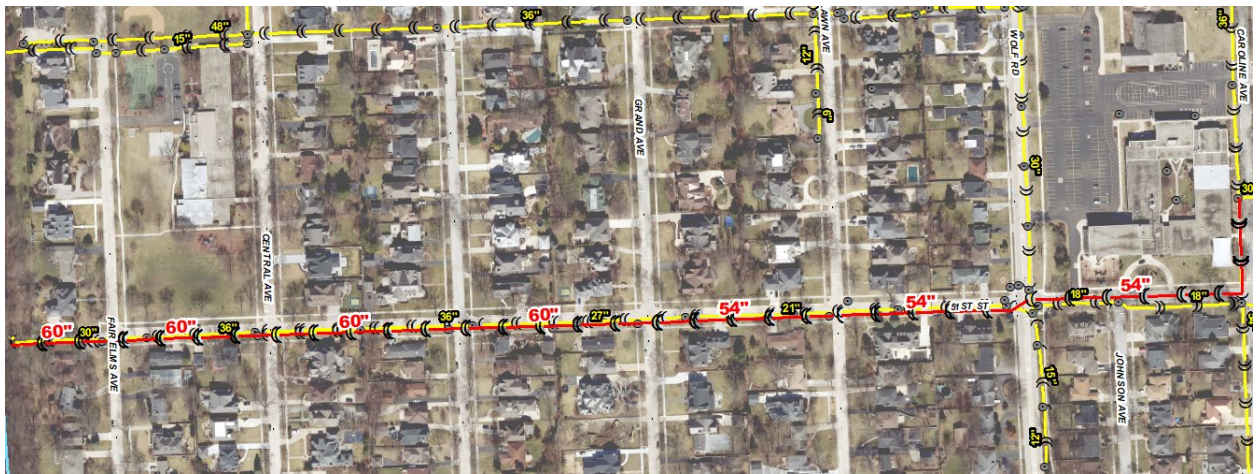
Figure 4. Upsized and New Storm Sewer on 51 st Street from Caroline Ave to Flagg Creek
