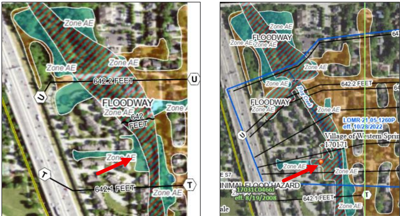
Figure 3: FEMA FIRMette before and after LOMR 21-05-1260P became effective on 10/28/2022. Approximate location of reverse siphon is shown with red arrow.
