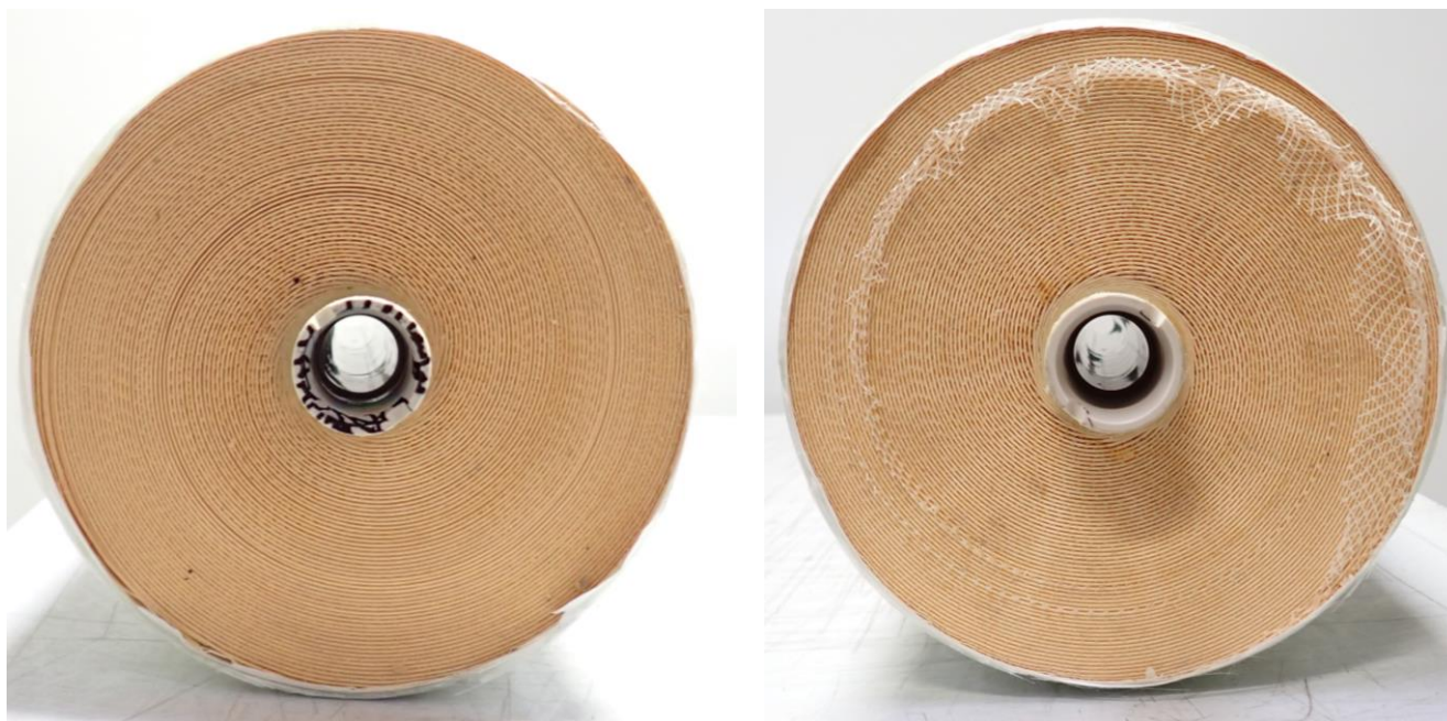
Feed (left) and concentrate (right) scroll ends of SN 2190531452
