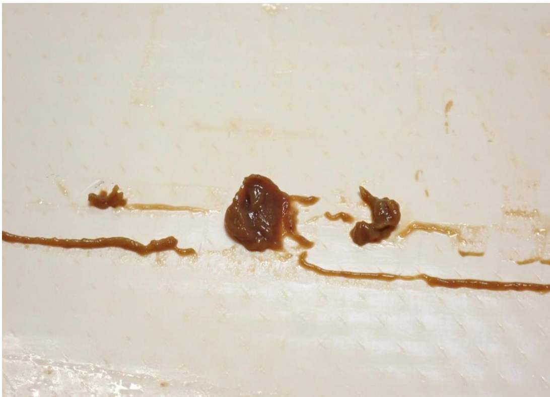
Foulant scraped on one membrane leaf of SN 2190531452
